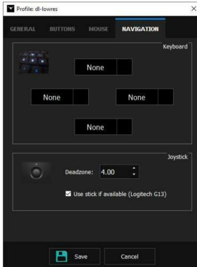
In case of Logitech G13, we have a mechanical joystick so a deadzone must be configured.
